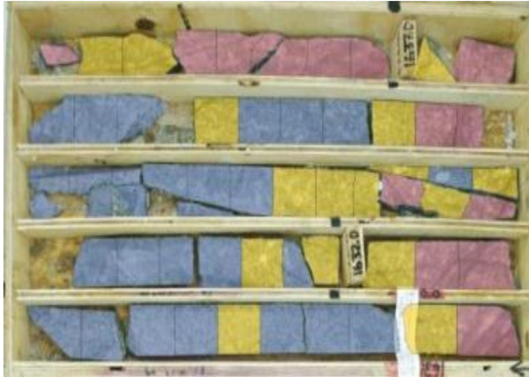
Core section from Hole 11-59 from 1630 to 1640 feet assayed 0.175% Mo
